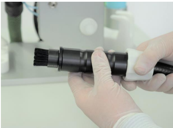
Attaching the suction nozzle
