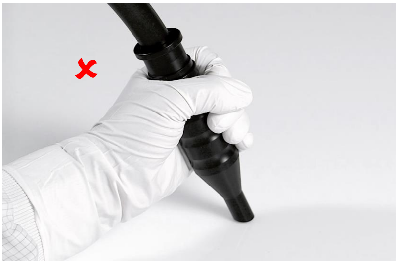
Incorrect distance and angle to hold the suction nozzle
