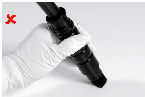
Applying the brush nozzle incorrectly
