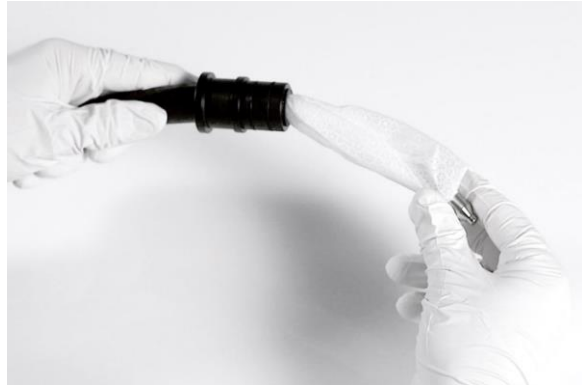
Alcohol-soaked cleaning cloth pushed through
