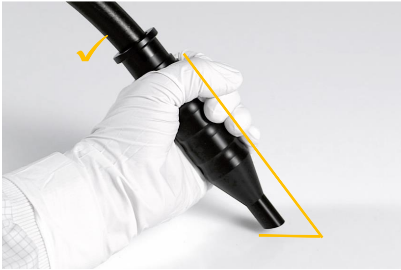
Correct distance and angle to hold the suction nozzle
