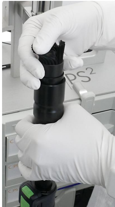
Pre-cleaning the brush suction nozzle mechanically
