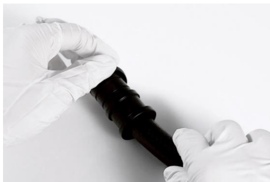
Covering hose ends with plugs
