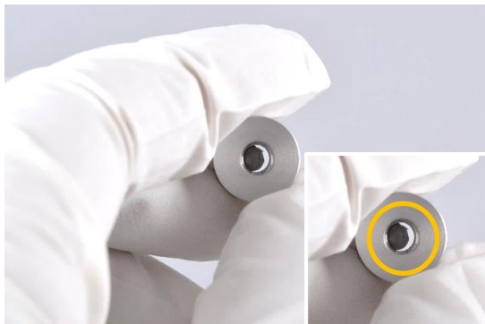
Blocked cone thread
