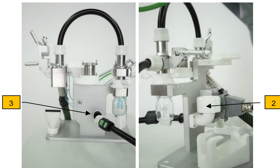
Determining the blank value, suction with prefilter via drying adapter
