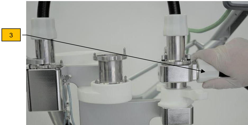
Attaching the suction hose (1 or 2 m)
