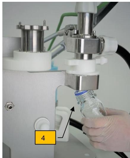
Replacing the particle collection jar
