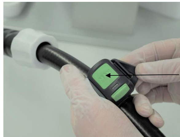
Attaching the Bluetooth remote control
