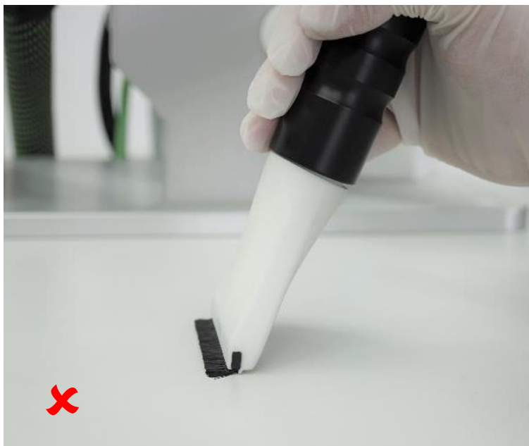
Applying the flat nozzle incorrectly
