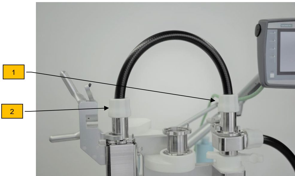
Interconnecting cyclone unit and filter unit
