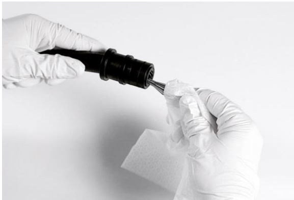
Alcohol-soaked cleaning cloth inverted by 180°
