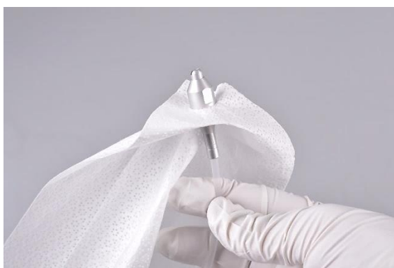
Cleaning wire with attached alcohol-soaked cleaning cloth
