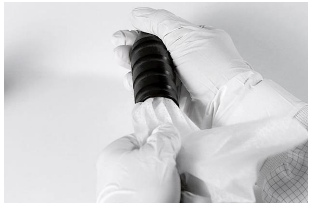
Cleaning the suction nozzle
